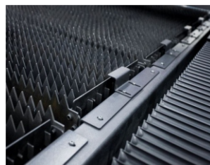
New support rack 5mm MS support rack over 4000W power machine
