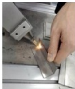
Angel welding, Erect welding
